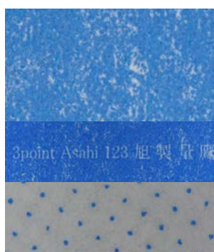
Standard hard type Flat Top plate print on paper based substrate. Solid, Reverse Text and 2% dot @ 150 lpi
