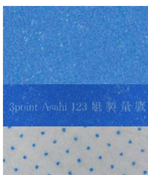
AWP™-CleanFlat Medium print on paper based substrate. Solid, Reverse Text and 2% dot @ 150 lpi
